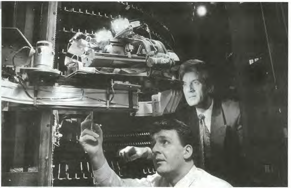
Above: Gary Newall, Storage Technology, making final adjustments to the robotic arm with Mike Gibbs, Computer Operations Manager, looking on. The circular design of the ATL can be clearly seen in the photograph with the 'empty' cartridge slots located around the inside. The 'eyes' of the robot are also in view — two bright lights above Gary. Picture by Mike Hall.
