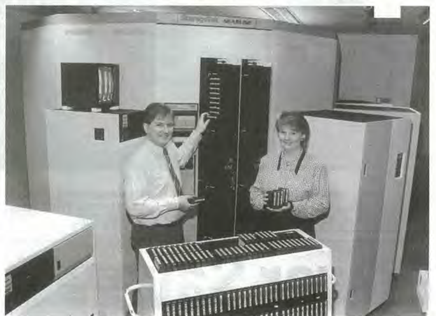
Above: Gary Newall, Storage Technology, making final adjustments to the robotic arm with Mike Gibbs, Computer Operations Manager, looking on. The circular design of the ATL can be clearly seen in the photograph with the 'empty' cartridge slots located around the inside. The 'eyes' of the robot are also in view — two bright lights above Gary. Picture by Mike Hall.
